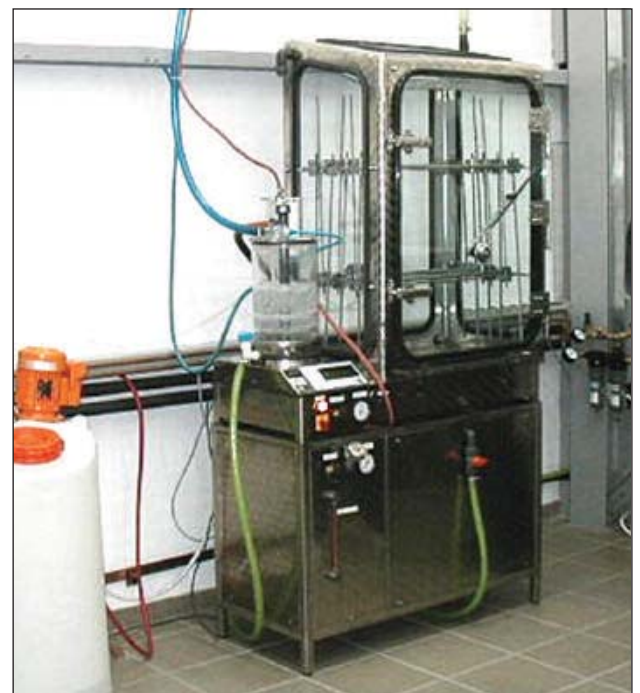
Environmental ageing chamber for ammonia atmosphere ageing
